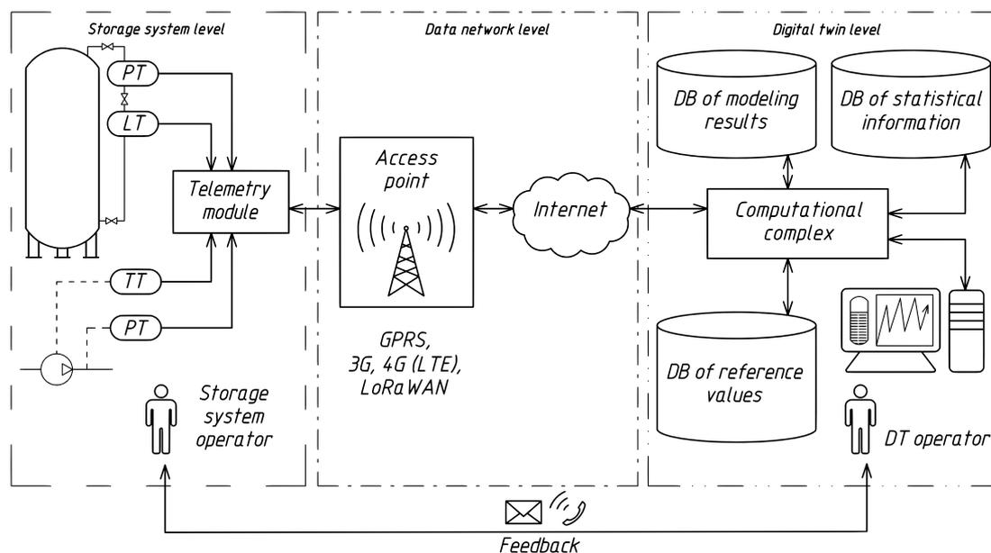
**Fig. 1.** Structure of the information system for monitoring the condition of cryogenic equipment (CS – storage system; DB – database; CD – digital twin; PT, LT, TT – transducers, respectively, pressure, level and temperature)
