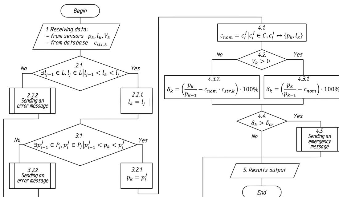
**Fig. 2.** Algorithm for calculating an assessment of the current technical condition of a vessel based on changes in the growth rate of cryoprodukt pressure
