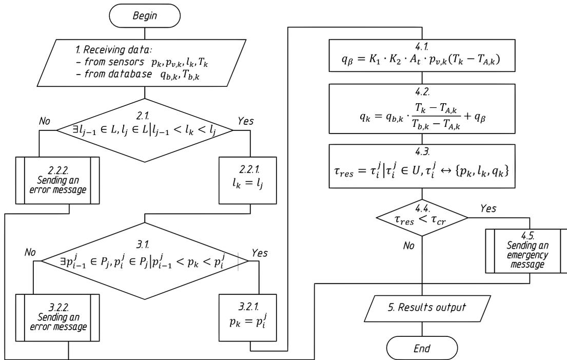
**Fig. 3.** Algorithm for calculating the time of non-drainage storage, taking into account changes in vacuum pressure in the thermal insulation cavity
