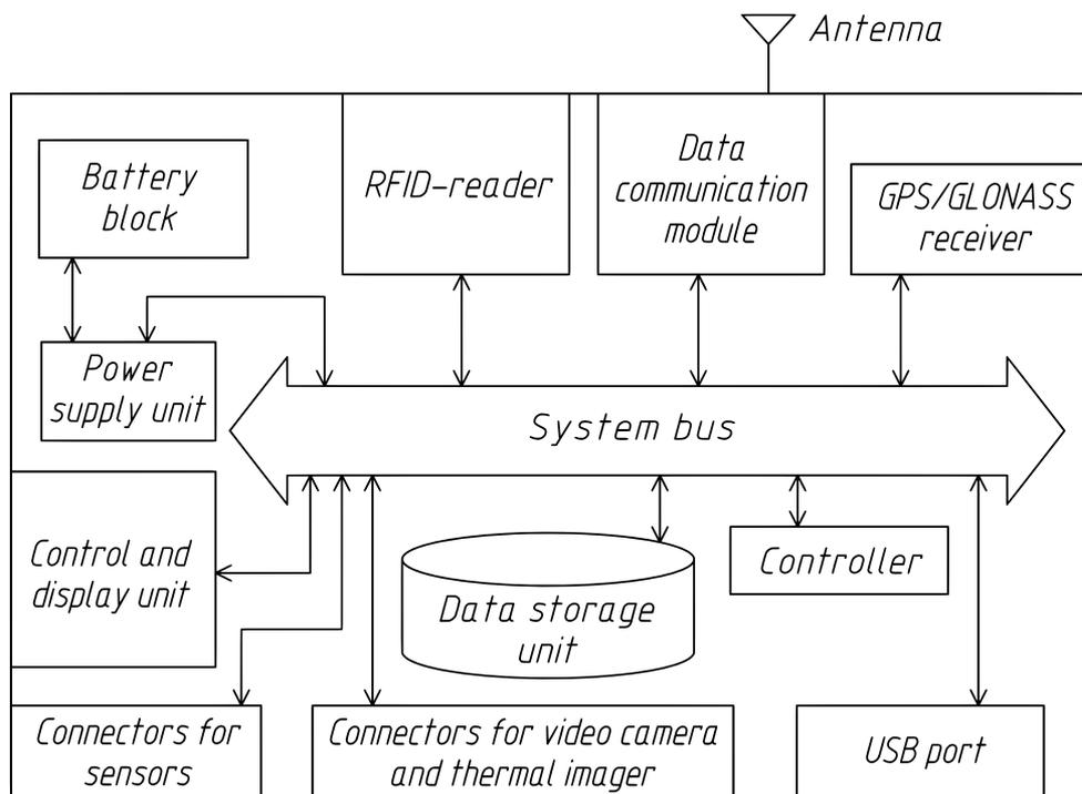
**Fig. 6.** UAV telemetry module for cryogenic equipment monitoring
