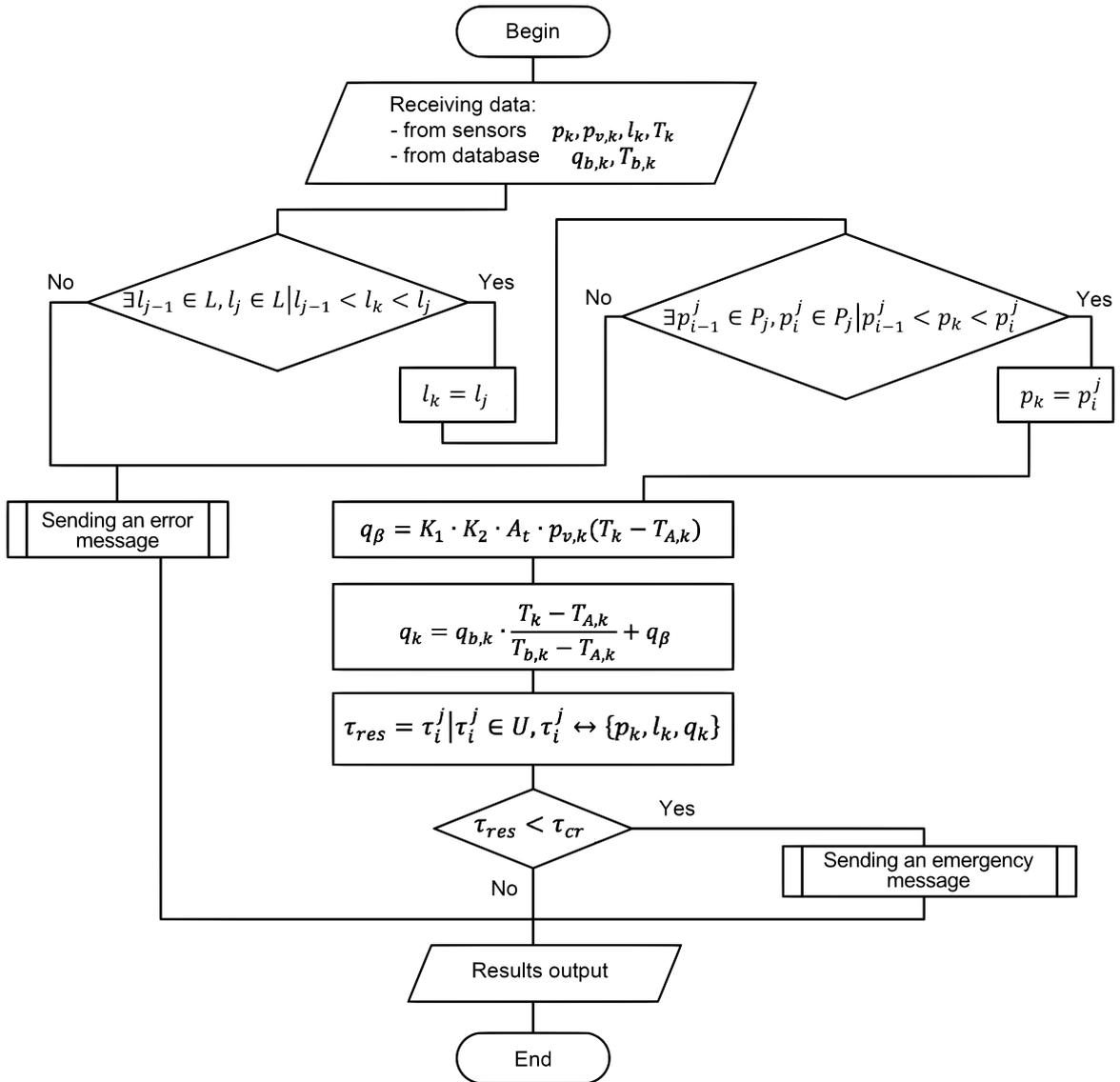
Fig. 4. Computational algorithm for storage time assessment by vacuum pressure deviation
