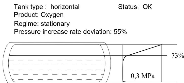
**Fig. 1.** Typical information picture for horizontal cryogenic tank
