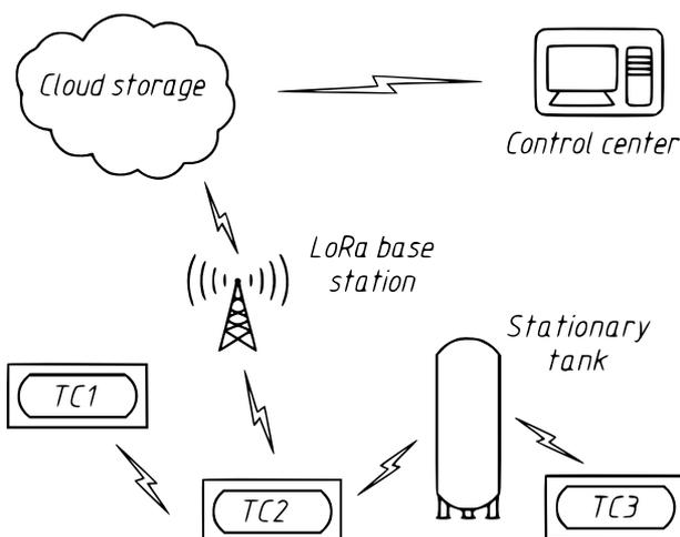
**Fig. 2.** Sensor network for monitoring the state of cryogenic equipment (TC1, TC2, TC3 – tank containers)
