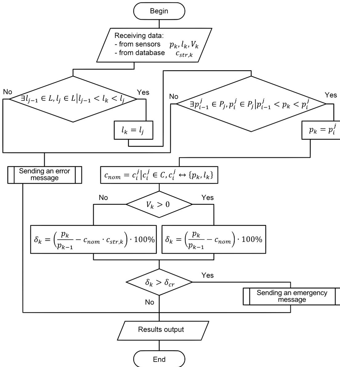
Fig. 3. Computational algorithm for condition assessment of the tank thermal insulation
