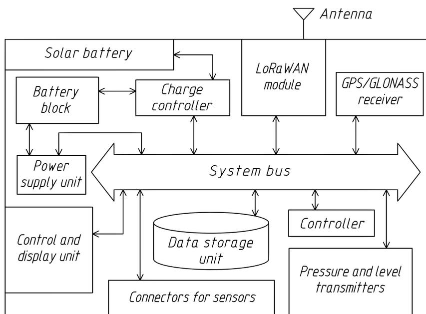
**Fig. 5.** Telemetry module for transport cryogenic equipment with autonomous power supply
