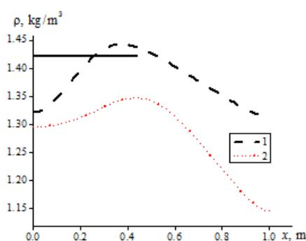
**Fig. 10.** Spatial distribution of gas density along the  $x$  axis ( $y = H/2$ ), curve 1 is a homogeneous gas, curve 2 is a gas suspension, straight line—analytical solution for inviscid gas
