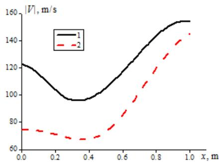
**Fig. 6.** Spatial distribution of the gas velocity modulus along the  $x$  axis ( $y = H/2$ ), curve 1 is a homogeneous gas, curve 2 is a gas suspension
