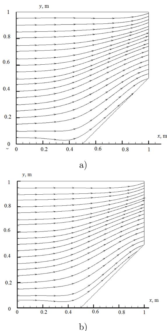
Fig. 2. Flowlines: a) in the carrier medium; b) in the dispersed phase
