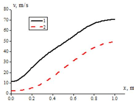
Fig. 8. Spatial distribution of the  $y$ -component of gas velocity along the  $x$  axis ( $y = H/2$ ), curve 1 is a homogeneous gas, curve 2 is a gas suspension
