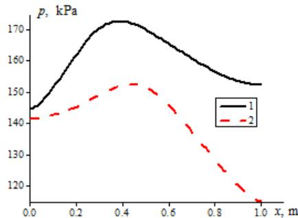
Fig. 9. Spatial distribution of gas pressure along the  $x$  axis ( $y = H/2$ ), curve 1 is a homogeneous gas, curve 2 is a gas suspension
