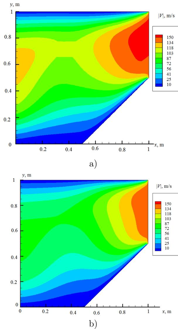
**Fig. 4.** Distribution of the modulus of velocity: a) of a homogeneous gas; b) of the carrier phase of the gas suspension
