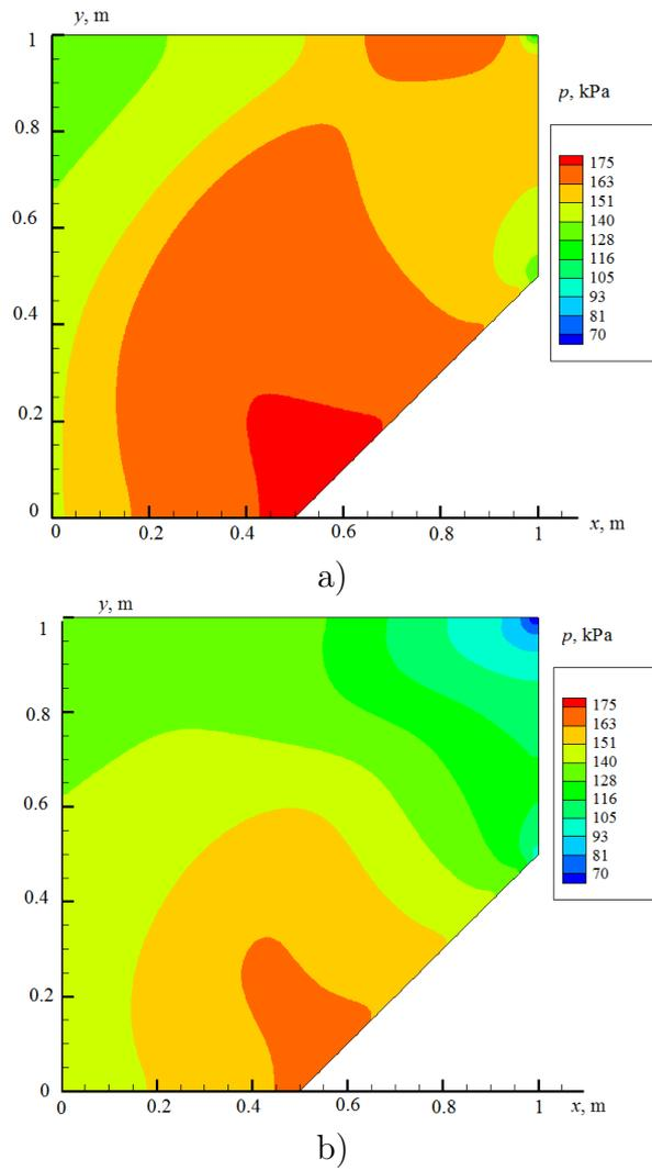
**Fig. 5.** Spatial distribution of pressure: a) of a homogeneous gas; b) of the carrier phase of the gas suspension
