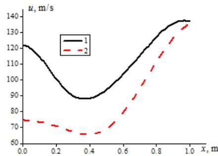
Fig. 7. Spatial distribution of the  $x$  component of gas velocity along the  $x$  axis ( $y = H/2$ ), curve 1 is a homogeneous gas, curve 2 is a gas suspension
