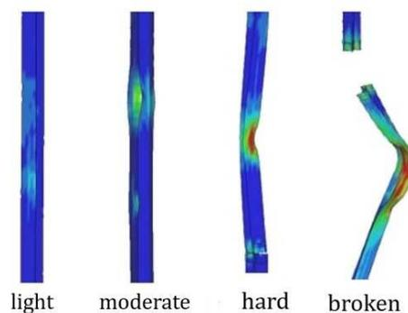
**Fig. 11.** Damage levels of the main columns
