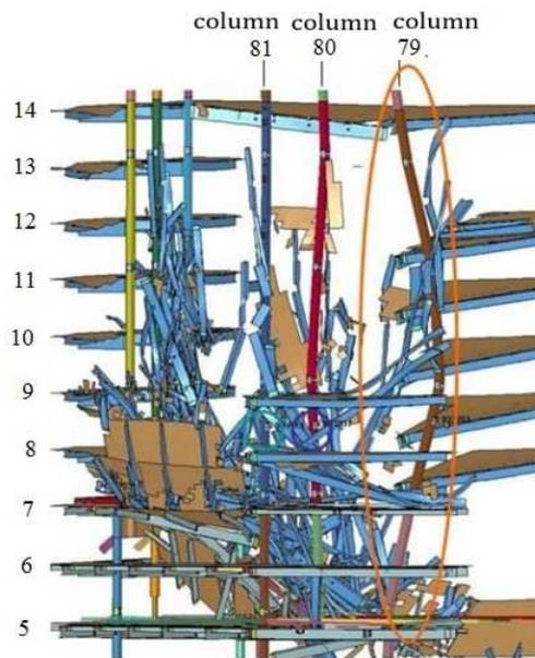
Fig. 12. The bend of column 79 to the east, when viewed from the southeast
