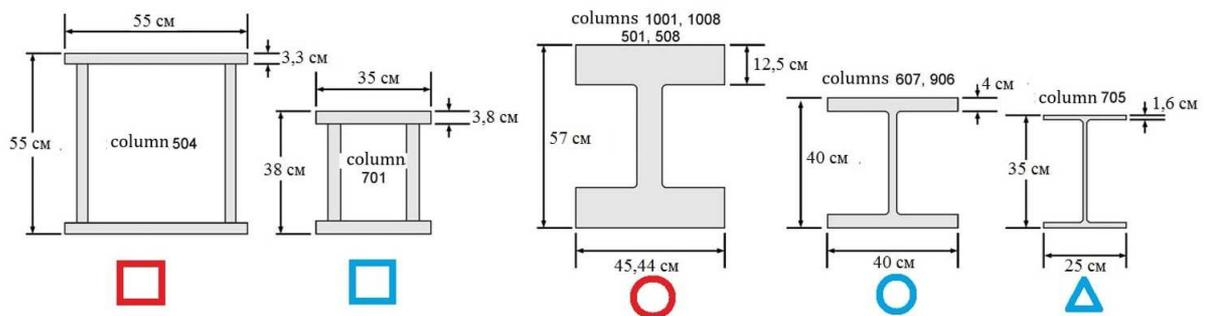
Fig. 5. Typical welded box elements and rolled wide shelves used for the main columns between the 83rd and 86th floors (in scale)
