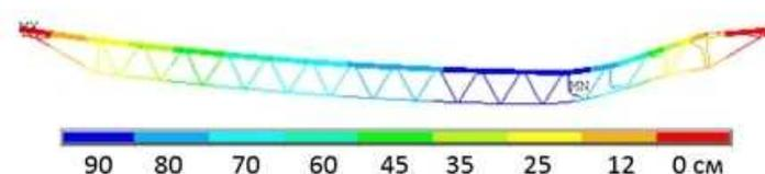
**Fig. 10.** Vertical displacement at  $700^{\circ}\text{C}$
