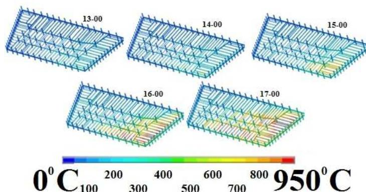
**Fig. 9.** Calculated temperature distribution ( $^{\circ}\text{C}$ ) of the 13th floor steel frame at five different points in time
