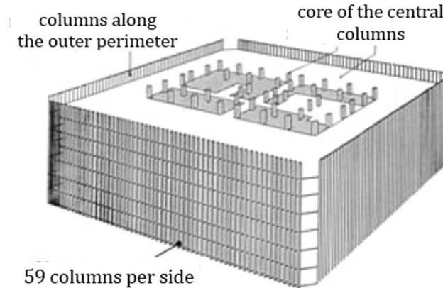
Fig. 2. The general structure of the floors of the twin towers
