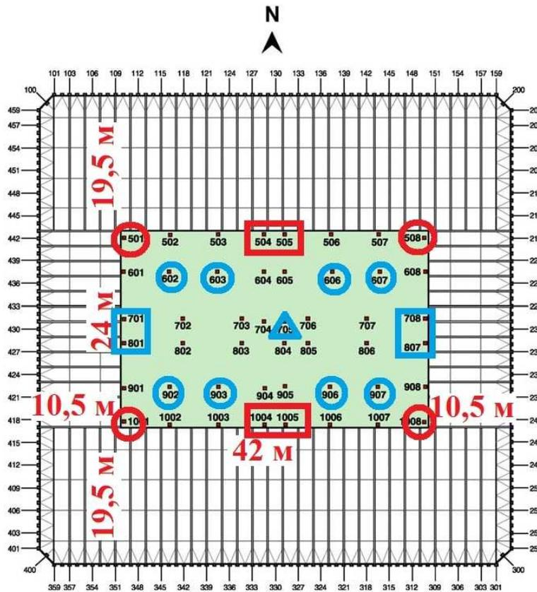
Fig. 4. Floor plan with indication of the types of column coupling
